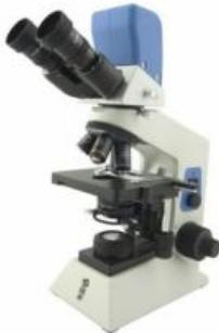
This binocular microscope has a built-in digital camera module, high resolution plan objectives and two wide field (WF) eyepieces with plan optics.
