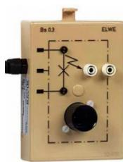
BS 0.3 Current-consuming equipment - "Filament lamp" The module is supplied by way of the service cable with grounding-type plug. The sockets located in parallel to the lamp symbol are used for the production of short-circuits to exposed conductive parts.
