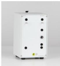
**BS 0.9 Transformer** The module includes an extra-low voltage and an isolating transformer. The mask specified below represents the corresponding graphic symbol in each case and covers the sockets which are not required. Primary: 230 V Secondary: 230 V, 42 V, 24 V, 90 VA
