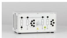
BS 0.2 Earthing Resistors This module includes all of the resistors required for the experiments. Resistance values: - Functional ground R<sub>b</sub>: 2 Ohm / 14 W - Protective ground R<sub>a</sub>: 2.2 Ohm / 11W, 220 Ohm / 220 W, 820 Ohm / 7 W, 1660 Ohm / 34 W - Potentiometer: 10k Ohm / 10 W with series resistor: 6.8k Ohm / 7 W - Insulation resistance R<sub>i</sub>: 15k Ohm / 2 W, 47k Ohm / 2 W, 82 kOhm / 2 W, 220 kOhm / 2 W Probe: 470 Ohm / 5 W
