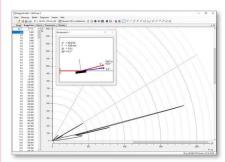
Bragg spectrum of a Mo anode on a NaCl single crystal in polar representation versus the sensor angle  $2\beta.$  The peaks in the diagram correspond exactly to the visible geometry in the X–Ray apparatus.
