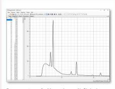
Bragg spectrum of a Mo anode on a NaCl single crystal versus the target angle  $\beta$ .
