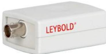
Plages de mesure :  $\pm 100/\pm 300$  pA,  $\pm 1/\pm 3/\pm 10/\pm 30/\pm 100/\pm 300$  nA,  $\pm 1/\pm 3/\pm 10$   $\mu$ A
