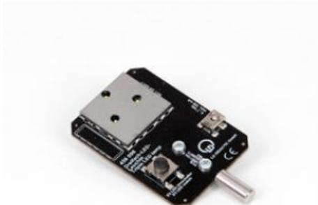
Triple LED lamp for student experiments to investigate additive and subtractive colour mixing.
