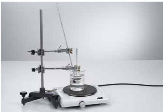
Determination of volumetric expansion coefficient of liquids (P2.1.2.1)
