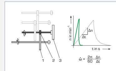
Determining the angular acceleration
