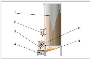
1 tube manometers, 2 tank for oil, 3 weight, 4 display and control unit for speed control, 5 measuring hoses, 6 journal bearing with drive
