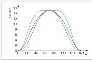
Elevation curves; s stroke,  $\alpha$  opening angle; blue: hollow cam, red: circular arc cam, green: tangent cam
