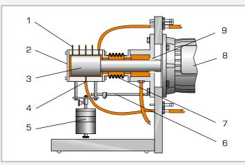
1 measuring points, 2 transparent bearing housing, 3 journal, 4 measuring point, 5 weight, 6 anti-twist device, 7 bellows, 8 drive motor, 9 radial sealing ring
