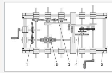
1 spur gear, 2 worm gear, 3 change gear, 4 Norton gear, 5 square steel tube frame
