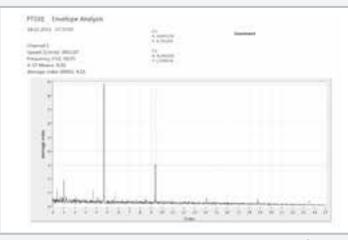
Envelope analysis of the bearing with damage on outer ring (B) at f=3000min<sup>-1</sup>
