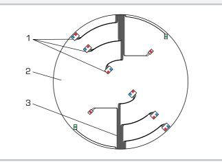
Strain gauge layout on the disk: 1 strain gauge measuring points, 2 disk, 3 wiring, red: strains in the radial direction; blue: strains in the tangential direction, green: shear
