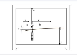
Bending on a cantilever beam: f draw down of the beam's end, x distance, a unloaded region with linear elastic line, b loaded region
