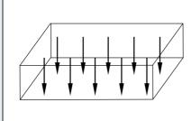
Volume force: acts spatially distributed over the volume of a body (weight, magnetic and electrical forces)
