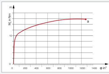
Torsion test of metallic materials to fracture:  $M_{t}$  twisting moment,  $\phi$  twisting angle, a specimen fracture
