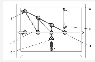
1 support with node disk, 2 cross arm for lateral stability of truss, 3 load application device with force gauge, 4 node disk, 5 dial gauge, 6 frame SE 112  $\,$
