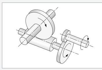
Drive principle of the two-stage helical worm gear
