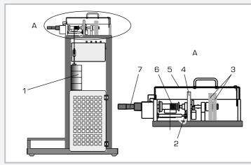
1 set of weights, 2 speed sensor, 3 flywheels, 4 drivegear, 5 protective cover, 6 cable drum, 7 hand crank
