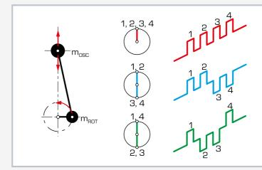
Left: definition of the rotating (m  $_{\rm ROT}$ ) and oscillating (m  $_{\rm OSC}$ ) masses at the crank drive, right: possible configurations of the crankshaft: red: single cylinder, blue: two-cylinder, green: four-cylinder
