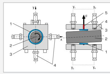
Sectional views of the journal bearing: 1 bearing shell, 2 shaft, 3 bearing housing, 4 displacement sensors (4 in X direction, 4 in Y direction), 5 oil supply, F load
