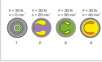
Effect of lubricating film thickness on speed: 1 static case, 2 to 4 increase in lubricating film width (lubricating oil ISO VG 100)
