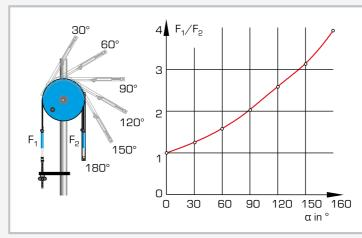
Gradual adjustment of the wrap angle from 30° to 180°. Diagram shows the force ratio  $F_1 / F_2$  as a function of the wrap angle  $\alpha$ .
