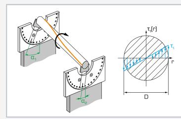
Torsion of a bar and measurement of the angles  $\alpha_1$  and  $\alpha_2$  right: shear stresses on the circular section
