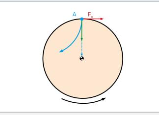
Effect of the Coriolis force: A starting point of the moving mass, F<sub>c</sub> Coriolis force; orange: rotating reference frame, red: direction of the Coriolis force, green: current motion of the mass, dashed blue: direction of movement without rotation, blue: actual direction of movement with rotation
