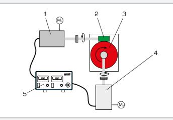
Determining the efficiency in the worm gear: 1 motor, 2 worm, 3 worm gear, 4 brake, 5 display and control unit;  $M_{\rm d}$  drive torque,  $M_{\rm b}$  braking torque
