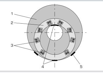
Strain gauge layout in cylinder wall and on the surface:
