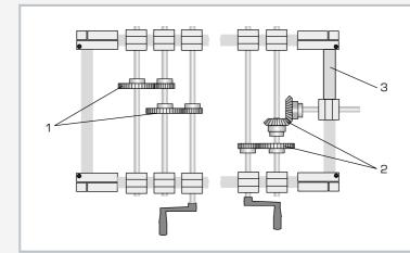
1 two-stage spur gear, 2 combined spur-bevel gear, 3 square steel tube frame
