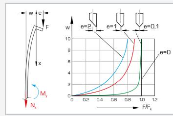
Experiment with eccentric application of force (WP 120.01): F applied force, e eccentricity, w deflection,  $M_y$  bending moment,  $F/F_k$  compressive force based on critical compressive force; diagram: deflection of the test bar for varying eccentricity
