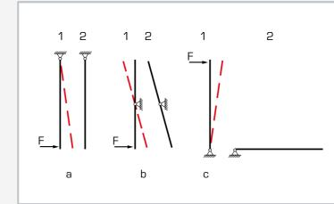
Various equilibrium positions: a stable, b indifferent, c unstable; position 1 deflection of the bar due to load, position 2 bar after load is removed
