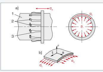
a) Strain gauge layout on the vessel: 1 vessel, 2 strain gauge measuring points, 3 wiring;  $\sigma_a$  stress in the direction of the vessel axis,  $\sigma_t$  stress in the circumferential direction,  $p_i$  internal pressure;
