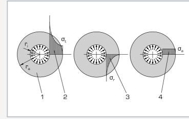
Distribution of stress in cylinder wall: 1 cylinder, r, inner radius, r, outer radius, 2 distribution of stress in hoop direction  $\sigma_{t}$ , 3 distribution of stress in radial direction  $\sigma_{r}$ , 4 distribution of stress in axial direction  $\sigma_a$
