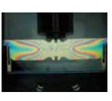
Top: model of a notched bar (FL 200.05) in monochromatic light, bottom: model FL 200.05 in white light
