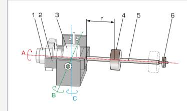
1 drive motor, 2 inner frame, 3 spinning top flywheel mass, 4 sliding weight, 5 lever, 6 fine weights; r distance of the weight, A horizontal axis of the spinning top = axis of rotation, B rotational axis of the inner frame = axis of gyro effect, C vertical axis = precession axis
