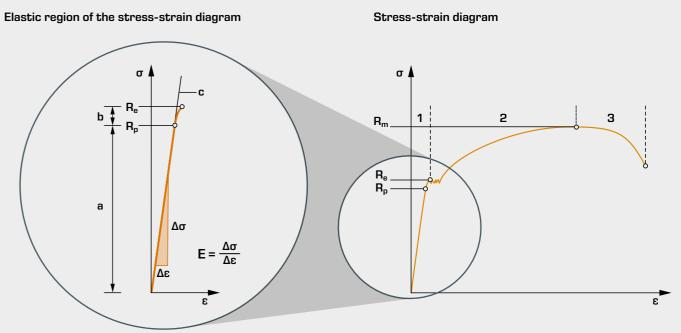
The elastic region is divided into a linear-elastic component a, where the strain is proportional to the stress and is reversible and a nonlinear-elastic component b, where the strain is not proportional to the stress but is still reversible. In the plastic region, the strain is not reversible and the deformation remains even after the force has been removed.
