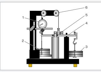
1 dial gauge, 2 balance weight, 3 weight, 4 loading plate, 5 test specimen in clamps, 6 deflection roller and cable to compensate for the dead-load of the plate
