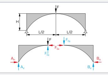
Top: symmetrically loaded three-hinged arch, bottom: free-body diagram of the loaded arch
