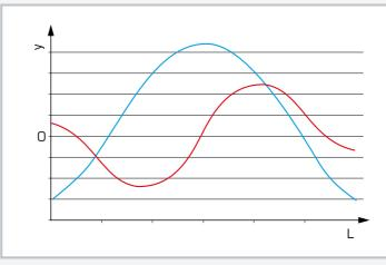
Elongation y of the vibration, shown over the length L of the model ship blue: first order natural frequency, red: second order natural frequency
