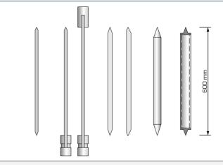
Test bars made of different materials and for different support types
