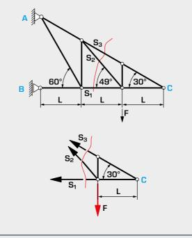
S bar forces,  $A\!+\!B$  support forces, C nodes, F force, L bar length,  $S_2$  wanted bar force
