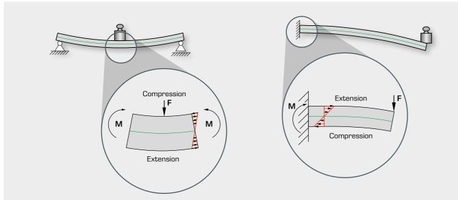
Tensile stress results in the extension of the outer strands, whereas compressive stress results in compression of the outer strands. The neutral strand (green) passes through the centroid and is neither compressed nor extended.
