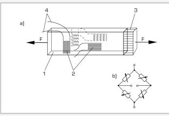
a) arrangement of strain gauges on tension bar, b) configuration of strain gauges; 1 tension bar, 2 strain gauge, 3 distribution of stress, 4 wiring; F applied force
