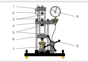
1 upper cross-member, 2 dial gauge for elongation, 3 clamp, 4 crosshead, 5 compression piece and pressure plate, 6 lower cross-member, 7 hydraulic cylinder, 8 hand wheel, 9 force gauge
