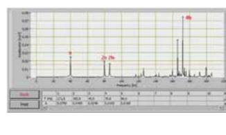
Typical spectrum of an electric motor rotary frequent vibration with n, 2n because of balance error power frequent vibration with 2fe, 4fe because of magnetic forces
