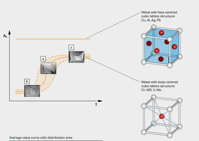
Ak notched-bar impact work, T temperature, a transition region (steep front) with mixed fractures, b depth position with low-deformation fractures, c height position with ductile fractures
