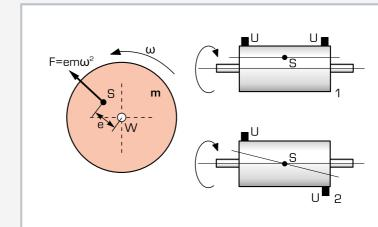
Left: imbalance force F due to eccentricity e of the centre of gravity S; 1 static imbalance with eccentric centre of gravity, 2 dynamic imbalance with inclined inertial axis; m mass, U imbalance, W axis of rotation,  $\omega$  angular velocity
