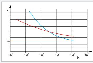
Woehler diagram for two different materials N: number of load cycles,  $\sigma$ : stress load on the specimer
