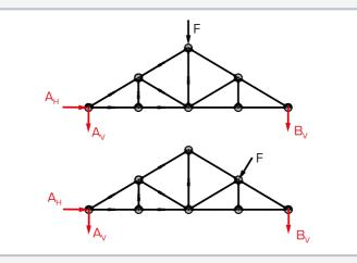
Load case, top: weight loading on ridge, load case, bottom: wind load perpendicular to roof; black: applied force, red: support reactions
