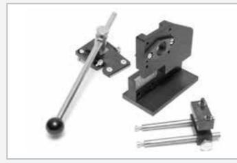
Functional groups of the lever shears: shear body, base, stop
