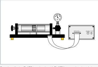
Example application: FL 152 in conjunction with FL 130 (stress and strain analysis on a thinwalled cylinder)
