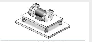
Imbalance generator on spring-loaded foundation
