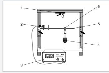
1 fixture, 2 strain gauge measuring point, 3 measuring amplifier, 4 weight, 5 bending bar, 6 adjustable ride
