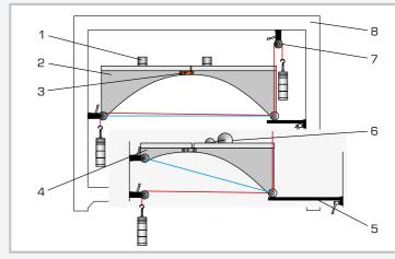
1 weight, 2 long arch segment, 3 crown hinge, 4 short arch segment, 5 support, 6 moving load, 7 deflection roller with fixture, 8 frame SE 112; red: cable, blue: springing line
