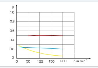
Coefficients of friction for different lubrication at constant load;  $\mu$  coefficient of friction, n speed, red: dry friction, blue: water lubrication, yellow: oil lubrication
