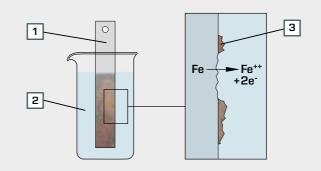
**Oxygen corrosion:** a direct electron exchange takes place between iron and oxygen-enriched water. The iron bonds with the oxygen to form iron oxide.
