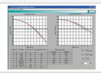
Application software for stress and strain analysis based on the example of the FL 120 (stress and strain analysis on a membrane)
