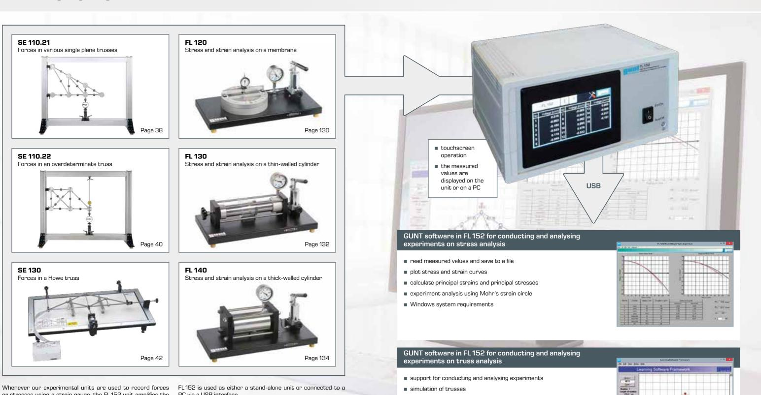
or stresses using a strain gauge, the FL152 unit amplifies the measuring signals. These signals are processed further and analysed using the GUNT software.
