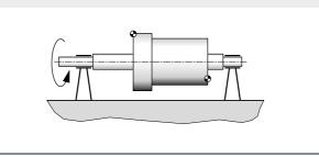
Rotor with points for mass balancing
