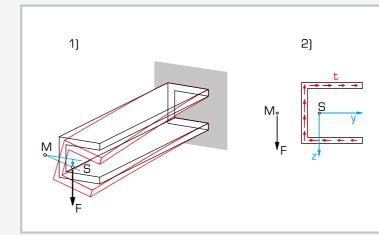
1 on application of the force at the centre of gravity the beam twists, 2 on application of the force at the shear centre no torsion occurs; M shear centre, S centre of gravity, F force, t shear flow
