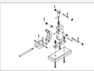
Exploded drawing of the lever press
