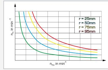
Curve of the precession speed for different gyroscopic moments  $n_{\mbox{\scriptsize Pr}}$  speed of the precession axis,  ${\rm n}_{\rm red}$  speed of the rotational axis,  ${\rm r}$  distance of the sliding weight (gives gyroscopic moment
