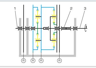
Principle of operation of a 2-stage planetary gear: 1 output shaft, 2 cable drum, 3 drive shaft, green: sun gears, yellow: planet gears, blue: ring gears, n speed
