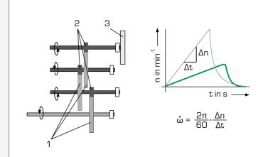
Determining the angular acceleration: 1 driving gears, 2 driven gears, 3 flywheel; speedtime diagram: determining the angular acceleration from the gradient of the curve
