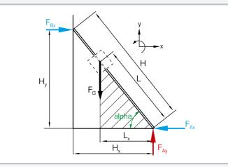
Free-body diagram of the leaning ladder: red: vertical support force, blue: horizontal support force, black: applied force
