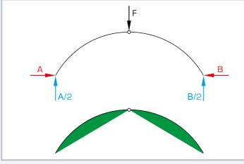
Theoretical bending moment curve in a symmetrically loaded arch: top: free-body diagram with calculated forces, bottom: qualitative bending moment diagram in green
