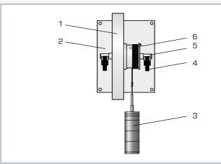
1 flywheel, 2 base plate, 3 weight, 4 bearing seat, 5 shaft, 6 cable drum
