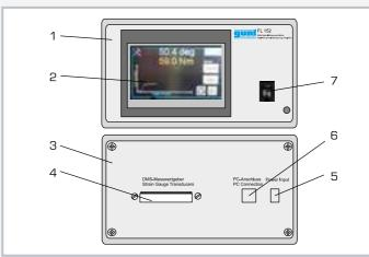
1 front view, 2 touchscreen, 3 rear view, 4 connection of strain gauge measuring points, 5 electric supply, 6 USB interface, 7 main switch
