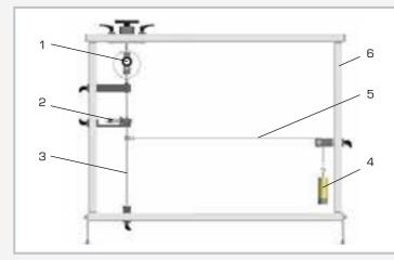
1 load mechanism, 2 dial gauges for lateral deflection of the sample bar, 3 test bar, 4 weight, 5 cable, 6 SE 112 mounting frame
