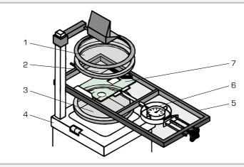
1 green filter, 2 analyser, 3 polariser, 4 overhead projector (FL 210.01), 5 frame, 6 load application device with force gauge, 7 plastic model
