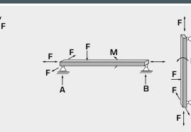
Bar: A support element, flexibly mounted at both ends, which can transfer tensile and compressive forces along the bar axis. Depending on whether a bar transfers tensile or compressive forces, it is referred to as a tension bar or a compression bar
