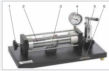
1 hand wheel for adjusting the piston, 2 vessel, 3 strain gauge measuring point, 4 manometer, 5 hydraulic cylinder with hydraulic pump, 6 port for FL 152 measuring amplifier
