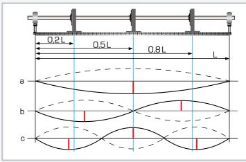
Natural modes of a shaft with continuous mass distribution: a) first natural mode, b) second natural mode, c) third natural mode; red: amplitude of the vibration, blue: position of the safety bearing; L clearance of the shaft bearing
