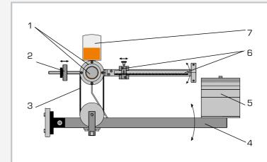
1 journal bearing housing with shaft journal, 2 tare weight, 3 belt to transfer force to the bearing housing, 4 loading lever, 5 weights, 6 measuring lever with scale and sliding weight, 7 drip oiler
