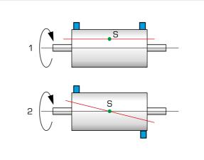
1 static imbalance, 2 dynamic imbalance; S centre of gravity; blue: mass distribution, red: principal axis of inertia
