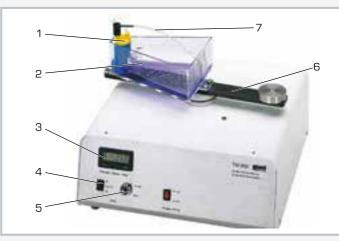
1 pump, 2 water tank, 3 speed display, 4 switch for direction of rotation, 5 speed adjustment, 6 rotating arm, 7 water jet
