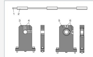
1 elastic shaft, 2 bearing, 3 safety bearing, 4 bores for displacement sensors, 5 bearing block with pendulum ball bearing, 6 bores for acceleration sensors
