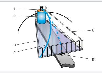
1 nozzle for water jet, 2 pump, 3 tank, 4 deflected water jet, 5 pivot point of the arm, 6 water jet with a stationary arm, 7 direction of rotation; A starting point of the moving mass
