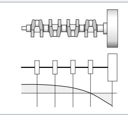
Crankshaft as an example of a torsional oscillator
