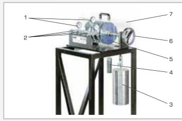
1 dial gauge, 2 bending beam, 3 set of weights, 4 set of weights for measuring transmission ratios, 5 planetary gear, 6 hand crank, 7 protective cover
