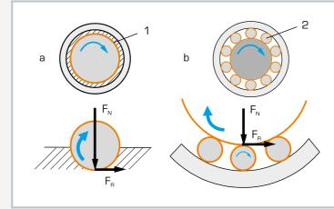
a dynamic friction in the slide bearing, 1 sliding surface
