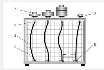
1 weight, 2 pinned support, 3 bar, 4 backing wall with grid pattern, 5 fixed support, 6 mount for weight
