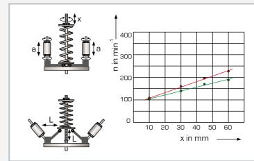
Settings and characteristic of the Hartnell governor at constant centrifugal force lever arm: a centrifugal mass adjustment, I centrifugal force lever arm, n speed, x spring preload; green increasing speed, red decreasing speed
