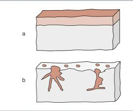
Two corrosion types: a surface corrosion, b pitting
