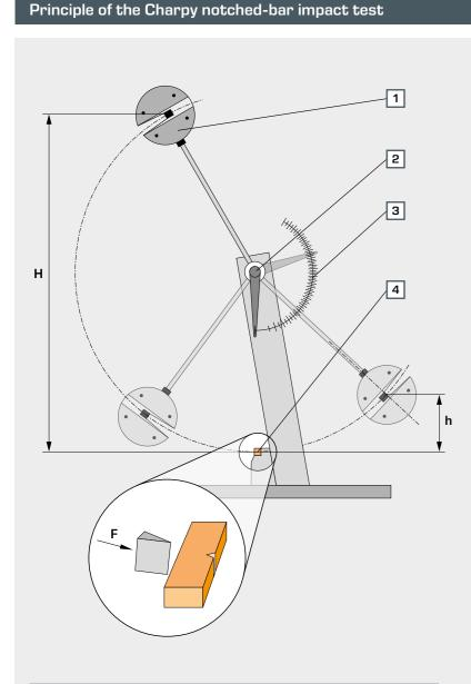
1 pendulum hammer, 2 axis of rotation, 3 scale with trailing pointer, 4 notched specimen; H height of fall, h height of rise, F force
