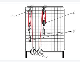
Experimental setup with the pulley blocks supplementary set (TM 110.02): 1 four-cable pulley block, 2 force gauge, 3 weight, 4 six-cable pulley block
