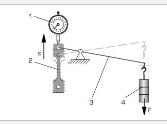
Principle of operation of the creep rupture test: 1 dial gauge, 2 specimen, 3 lever for load transfer, 4 weight; F force,  $\epsilon$  strain
