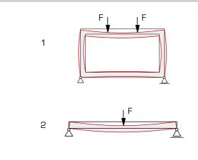
Suggestions for your own tests with various large components, for example 1 load on frame, 2 load on beam or girder
