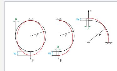
Deformations on curved-axis beams under tensile load: F force, r radius, u horizontal displacement, w vertical displacement
