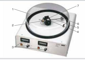
1 protective cover, 2 gyro drive motor, 3 speed displays and adjustment for of the horizontal gyro axis and the vertical precession axis, 4 spinning top flywheel mass, 5 lever, 6 sliding weight, 7 inner frame
