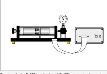
Example application: FL 152 in conjunction with FL 130 (stress and strain analysis on a thinwalled cylinder)
