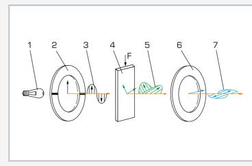
Schematic representation of the photoelastic demonstration: 1 light source, 2 polariser, 3 linear polarised light, 4 model under load, 5 light decomposed into two components in the directions of the principal stresses, 6 analyser, 7 horizontal components of the light
