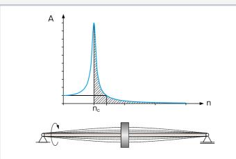
Vibration behaviour of a Laval rotor: n speed, A amplitude,  $n_{\rm c}$  critical speed with resonance, shaded area: subcritical speed, red shaded area: supercritical speed with self-centring
