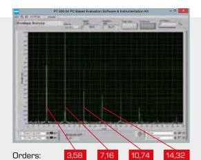
The illustration shows the envelope spectrum of typical bearing damage. To obtain a display that is independent of rotation frequency, the order was chosen as the abscissa. A rotational frequency signal is of the first order. Frequency lines are read in multiple of the order 3,58. This indicates damage to the outer ring of the bearing. The absence of first-order sidebands indicates a constant force direction, i.e. belt tension in this case, and no rotating imbalanced load.
