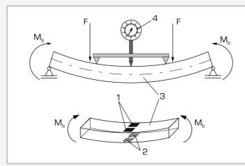
1 strain gauge on top of bar (compression side), 2 strain gauge on underside of bar (tension side), 3 bending bar, 4 dial gauge; M <sub>b</sub> bending moment, F applied force
