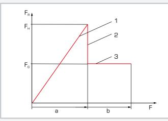
Frictional force at static and dynamic friction: 1 static friction, 2 slide limit, 3 dynamic friction,  $F_{R}$  frictional force, F traction,  $F_{H}$  static frictional force,  $F_{G}$  dynamic frictional force, a rest state, b motion
