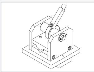
3D representation of the assembled bending device
