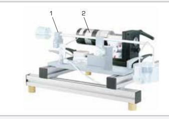
1 TM 260.05 experimental unit studies a tribological system, consisting of a cylindrical pin and a roller, which slide against each other (point contact), 2 TM 260 drive unit
