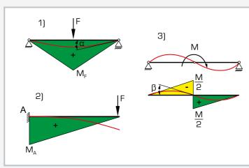
Bending moment characteristic (green/yellow) and elastic line (red) for statically determinate beams: 1 single-span beam with mid point load, 2 cantilever beam with point load, 3 single-span beam with bending moment as load;
