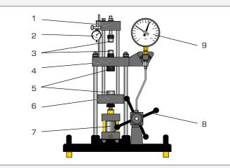
1 upper cross-member, 2 dial gauge for elongation, 3 clamp for tensile specimens, 4 crosshead, 5 compression piece and pressure plate, 6 lower cross-member, 7 hydraulic cylinder, 8 hand wheel, 9 force gauge
