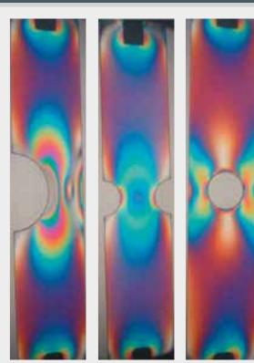
Tensile load with stress concentration on cross-sectional contraction
