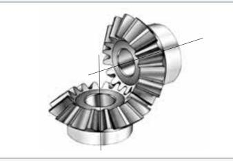
Bevel gear: drive and driven shaft at 90 degrees to each other. The outer form of the gear wheels (envelope) is equivalent to cones. The central axes intersect.
