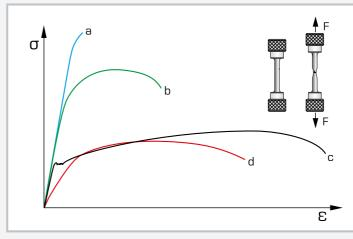
Stress-strain diagram for various materials: a hardened steel, b tempered steel, c annealed steel, d alloyed aluminium
