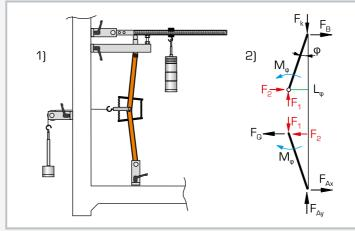
1) experimental setup for elastic joint with transverse loading
