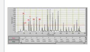
Frequency spectrum on the belt drive belt frequency  $f_{\rm r}$  with harmonic waves  $2f_{\rm r},\,4f_{\rm r},\,6f_{\rm r}.$  drive speed n, n/2
