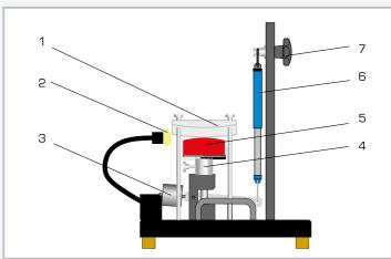
1 double convex plexiglas disk, 2 halogen lamp, 3 sliding weight to compensate the mass of the load mechanism, 4 load mechanism, 5 rubber pressure pad with convex surface, 6 spring balance, 7 movable device for the spring balance
