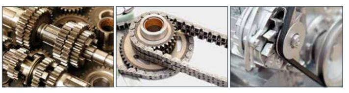
Complex machine elements used to alter the motion variables of path, velocity and acceleration are known as conversion elements or gears. In a gear drive, positively locking gears transfer the rotary motion from one shaft to another. In a traction drive, the rotary motion is transferred between two shafts by
