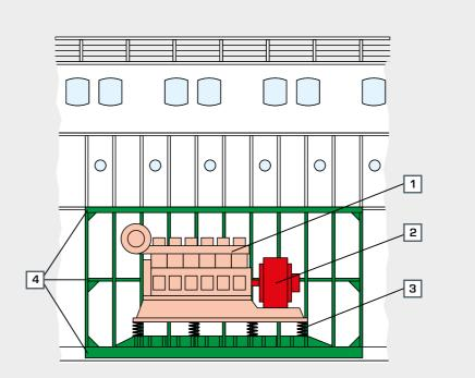
Minimising undesired vibrations using the example of a ship's engine system:
