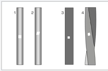
Deformation of a rectangular surface element (white): 1 round bar, not deformed, 2 round bar, twisted, 3 square tube, not deformed, 4 square tube, twisted
