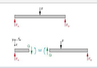
Internal forces on the beam under mid point load: F applied point load,  $F_A/F_B$  reactions (0,5F), Q shear force, M bending moment
