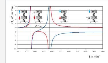
Amplitude-frequency response at unbalance excitation and effect of vibration absorbers m: mass, blue amplitude x1: mass 1, red amplitude x2: mass 2, A: absorption point
