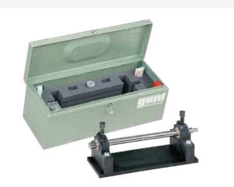
The illustration shows the tool box with the assembly kit and, in the foreground, the fully assembled journal bearing
