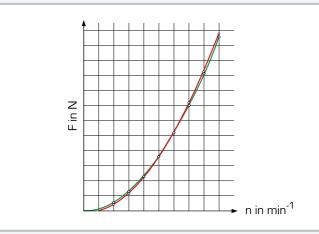
Dependence of centrifugal force on the speed green: calculated values, red: measured values; F centrifugal force, n speed
