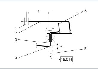
Principle of force measurement with force-proportional deformation:
