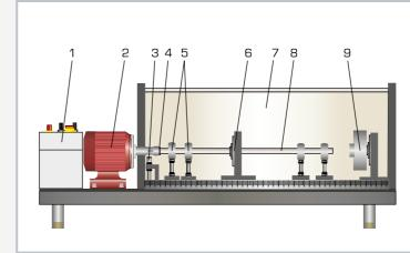
1 switch box, 2 motor, 3 inductive speed sensor, 4 elastic coupling, 5 self-aligning ball bearings, 6 safety bearing, 7 protective cover, 8 shaft, 9 mass disk
