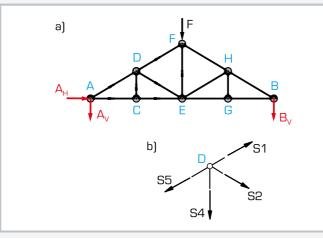
Free-body diagram of a truss, nodal section method: a) layout, black: applied force, red: support reactions, blue: node; b) bar forces at node D
