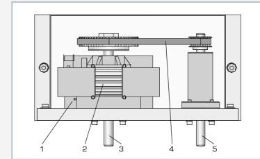
1 magnetic particle brake, 2 fan, 3 shaft for direct connection of brake, 4 belt drive, 5 shaft for connection of brake via belt drive
