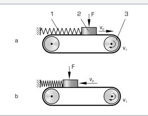
Friction oscillations (Slip-stick phenomenon): 1 spring, 2 body, 3 drive; F force, v velocity, a static, b dynamic
