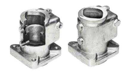
Machined (left) and raw casting (right)
