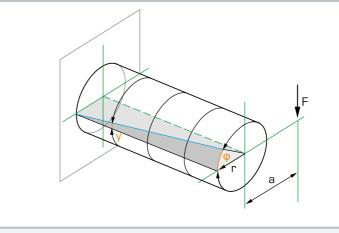
Torsion on round bar: F applied force, a lever arm, r radius, y shear angle,  $\phi$  angle of twist
