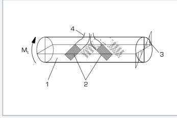
Arrangement of strain gauges on torsion bar: 1 round bar, 2 strain gauge, 3 distribution of stress, 4 wiring;  $M_{\rm t}$  torque
