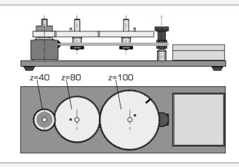
Experimental setup with locked rail and two additional axles
