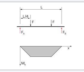
Force and bending moment characteristic on the bending bar: black: applied force, red: support reactions
