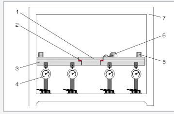
1 suspended beam, 2 articulated support, 3 cantilever beam, 4 support with force gauge, 5 weight, 6 moving load, 7 frame SE 112
