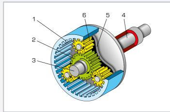
Layout of a planetary gear: 1 ring gear, 2 sun gear, 3 sun gear shaft, 4 planet carrier shaft, 5 planet carrier, 6 planet gear
