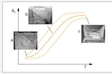
Notched bar impact work-temperature diagram with typical fracture surfaces: averagevalue curve with distribution area, Ak notched bar impact work, T temperature; a depth position with low-deformation fractures, b transition region (steep front) with mixed fractures, c height position with ductile fractures
