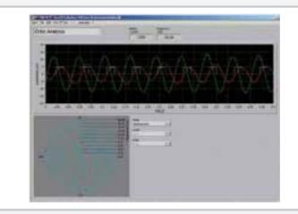
Screenshot of evaluation software above: vibration signals as a function of time below: orbit view for vibration on two planes
