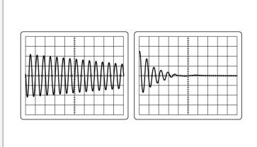
Example oscillograph: left - torsional vibration of a torsion bar with mass disk, weakly damped; right - the same vibration with strong damping
