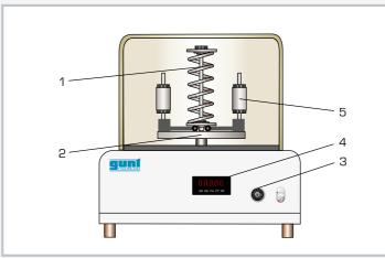
1 spring, 2 Hartnell governor centrifugal system, 3 control element for adjusting speed, 4 speed display, 5 centrifugal mass
