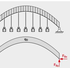
Line load and support reactions on an arch
