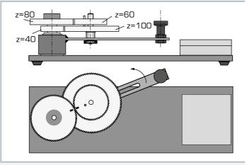
Experimental setup with unlocked rail and one additional axle Planetary gear: driven wheel (40 teeth) coupled to the fixed axle, driven via rail, rail as planetary gear, planetary wheels (100 teeth, 60 teeth), sun wheel as driven wheel (80 teeth)
