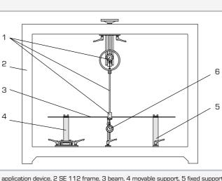
1 load application device, 2 SE 112 frame, 3 beam, 4 movable support, 5 fixed support, 6 dial gauge
