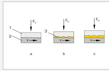
Effect of the lubricating film on friction: 1 pin, 2 disk, 3 lubricant; a dry friction, b mixed friction, c fluid friction;  $F_N$  force, v velocity
