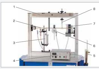
1 pendulum bearing, 2 bar-type oscillator, 3 container for oil damper, 4 control unit for imbalance exciter, 5 storage for additional pendulums, 6 imbalance exciter, 7 drum recorder, 8 spring
