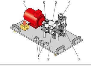
1 interchangeable cam-shaped cam member, 2 nib, 3 spring, 4 mass disks, 5 flywheel, 6 recorder drum, 7 drive motor
