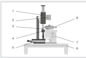
1 reflected light microscope, 2 halogen lamp, 3 steel sphere, 4 load application device, 5 cross table, 6 frame of TM 260, 7 drive unit from TM 260, 8 glass plate
