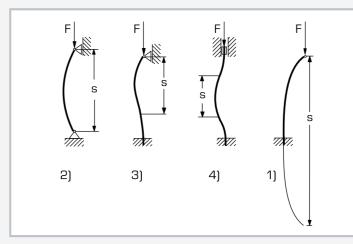
Buckling length dependent on end conditions of bars: 1) Euler case 1: fixed-free bar 2) Euler case 2: pinned-pinned bar 3) Euler case 3: fixed-pinned bar (pinned at the top) 4) Euler case 4: fixed-fixed bar; F applied buckling load, s buckling length
