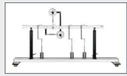
WP 960 Beam on two supports: shear force & bending moment diagrams
