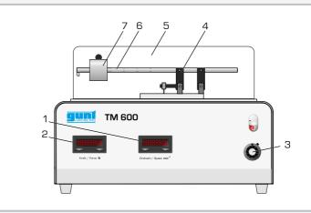
1 centrifugal force display, 2 speed display, 3 adjustment of the speed, 4 connecting rod (force measurement), 5 protective cover, 6 rotating arm, 7 mass
