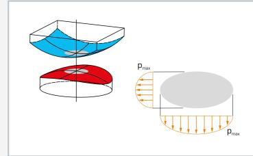
Contact area between two bodies with curved surfaces; grey: contact area in the shape of an ellipse, orange compressive force (pressure)
