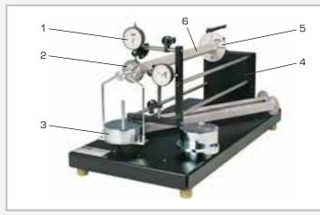
1 dial gauge, 2 device to adjust the eccentricity of the load application point and flange to mount the load, 3 weight, 4 clamping pillar, 5 clamping flange of beam with angle scale, 6 beam
