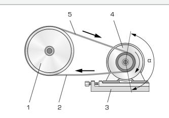
How a belt drive works: 1 driven pulley, 2 slack span, 3 tensioning rail with screws, 4 drive pulley. 5 tight span: α wrap angle
