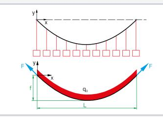
Substitute model for a suspension bridge: "suspended cable with uniformly distributed load" with free-body diagram (bottom); F cable force,  $q_0$  distributed load; f maximum sag, L span
