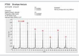
Envelope analysis of the bearing with damage on outer ring (B) at f=1800min<sup>-1</sup>, damage frequency f<sub>1</sub>=3,58f, harmonic waves f<sub>2</sub> to f<sub>7</sub>
