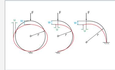
Deformations on curved-axis beams under compressive load: F force, r radius, u horizontal displacement, w vertical displacement
