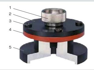
Assembled drilling jig with workpiece: 1 fastening screw, 2 drill plate, 3 drill bush, 4 workpiece (bearing cap), 5 base
