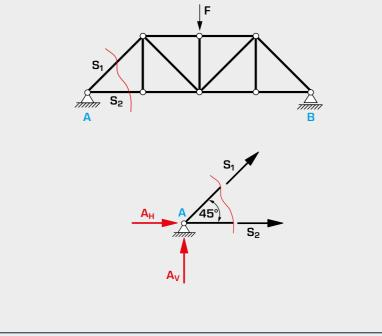
S bar forces, A+B support forces, F forces, index V vertical forces, index H horizontal forces
