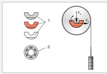
1 interchangeable bearing shells of cast iron, red bronze and plastic (PTFE), 2 roller bearing; F<sub>N</sub> normal force, F<sub>R</sub> frictional force
