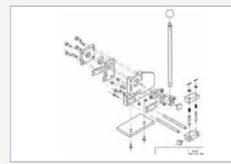
Exploded drawing of lever shears
