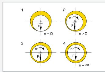
Operation of a hydrodynamic journal bearing: 1 to 4 build-up of a load-bearing oil film at increasing speed
