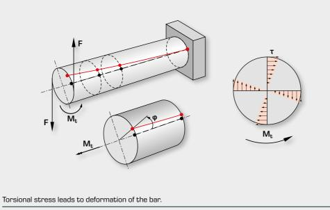
$M_t$  twisting moment, F force,  $\phi$  twisting angle,  $\tau$  shear stress
