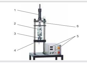
1 hydraulic cylinder for generating tensile and compressive forces, 2 operating area with the accessory WP 310.05, 3 force sensor, 4 adjustable height lower cross-member with lock, 5 displays and controls, 6 displacement sensor
