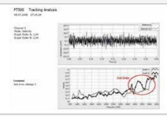
Tracking analysis of a rotor with crack: significant rise in amplitude in 2 <sup>nd</sup> order (marked red)
