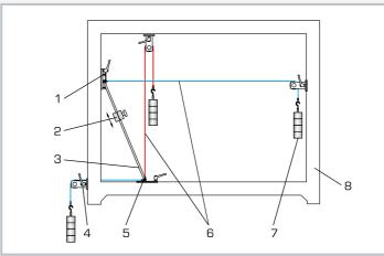
1 support (movable support), 2 clamp weight, 3 ladder, 4 clamp guide pulley, 5 support (fixed support), 6 cable, 7 weight, 8 SE 112 mounting frame
