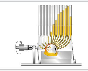
Pressure distribution over the bearing shell; pressure increases as the bearing gap decreases
