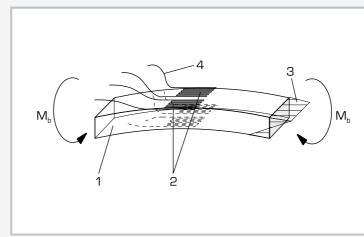
Arrangement of strain gauges on bending bar: 1 bar, 2 strain gauge, 3 distribution of stress, 4 wiring;  $M_{\rm b}$  bending moment
