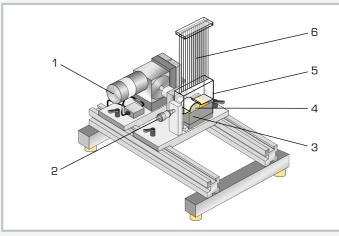
1 TM 260 base module, 2 bearing gap width adjustment, 3 oil pan, 4 shaft, 5 bearing housing with bearing shell, 6 tube manometers
