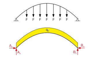
Top: forces on the statically indeterminate parabolic arch,
