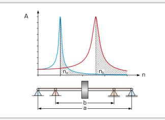
Reducing the bearing clearance increases the critical speed; A amplitude, n speed; n<sub>a</sub> critical speed at bearing clearance a, n<sub>b</sub> critical speed at bearing clearance b, shaded area: supercritical speed
