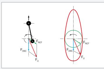
Left: effect of the oscillating (blue, F<sub>OSC</sub>) and the rotating (green, F<sub>ROT</sub>) mass forces and their vectorial addition to the free mass force (red,  $F_{U}$ ). Right: mass forces course during a crankshaft revolution
