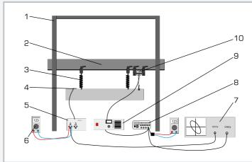
1 frame, 2 adjustable height cross-member, 3 springs for suspending the model ship, 4 acceleration sensor, 5 measuring amplifier, 6 multimeter, 7 oscilloscope (not included) 8 function generator, 9 power amplifier for vibration exciter, 10 vibration exciter
