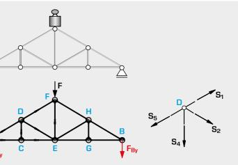
Method of joints to determining the forces on a truss F force, F<sub>Ax</sub>, F<sub>Ay</sub>, F<sub>By</sub> support forces, S bar forces, A-H joints
