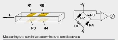
R2 + R4 measurement of longitudinal strain,
