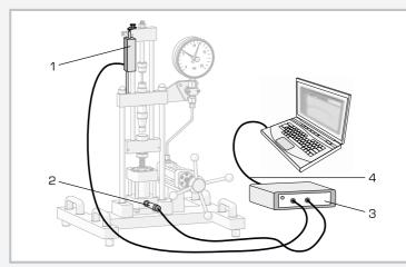
Port for connecting data acquisition to the basic unit: 1 displacement sensor, 2 pressure sensor for force measurement, 3 measuring amplifier, 4 USB cable
