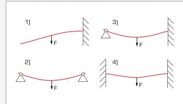
Beam deflection of a statically determinate (left) and indeterminate (right) system: 1 cantilever beam, 2 simply supported beam, 3 propped cantilever, 4 built in beam
