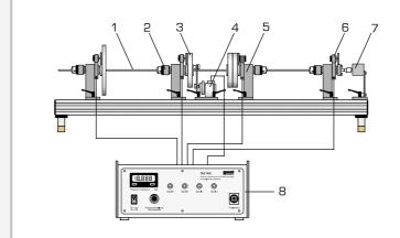
1 torsion bar, 2 clamping chuck, 3 mass disk, 4 exciter unit, 5 bearing unit, 6 rotary angle sensor, 7 damper unit, 8 display and control unit
