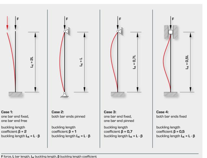
To determine the buckling stress we use the degree of slenderness  $\lambda$  as a material parameter and the moment of area radius i.
