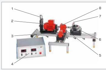
1 spring balance, 2 motor, 3 worm gear, 4 display and control unit, 5 spur gear, 6 brake, 7 brake lever arm, 8 coupling
