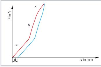
Load-extension diagram for red: load curve and blue: relief curve; a elastic region, b region of non-linear deformation, c plastic range, d permanent deformation; F force, s elongation
