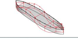
Second order natural frequency of a ship's hull
