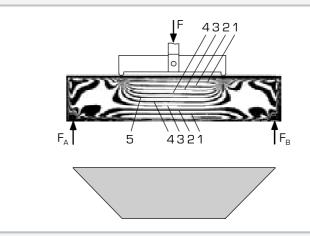
Top: stress distribution in the model under bending load: 1 to 4 isochromat layout, 5 neutral strand; F external force,
