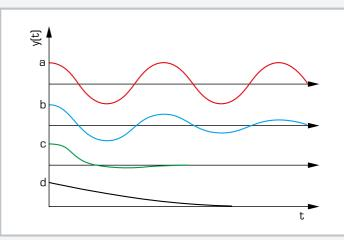
Modes of vibration for varying damping D: a) no damping, D = O, continuous vibration, b) low damping, O < D < 1, c) D=1, aperiodic limit case, d) strong damping, D > 1, creep case; y elongation, t time
