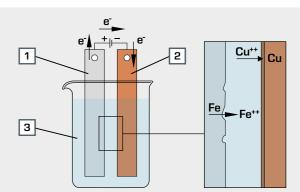
Electrochemical corrosion occurs through the formation of galvanic elements. If two different metals come into contact, an electrical current flows in the presence of an electrolyte. This dissolves base metal. More or less current flows depending on the metals present, and destruction takes place.
