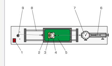
1 mains power switch, 2 carriage, 3 friction body, 4 additional weight, 5 supporting friction surface, 6 damping cylinder, 7 force gauge, 8 guide, 9 drive motor with cable drum
