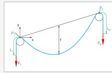
Actual applied cable forces:  $F_1 + F_2$  forces,  $L_1 + L_2$  suspended chain length with deadweight,  $P_1 + P_2$  marker point on chain wheel, f sag
