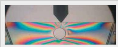
Bending load with central force and cross-sectional contraction
