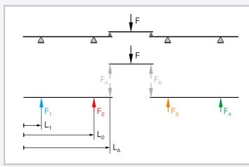
Top: simplified experimental setup (Gerber beam), bottom: free-body diagram: F applied force,  $F_A + F_B$  reactions of the articulated supports,  $F_1...F_4$  reactions of the supports with force gauge,  $L_1$ ,  $L_2$ ,  $L_A$  positions of the supports
