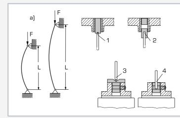
a) experiment on how bar length affects the buckling behaviour:
