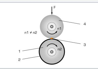
Tribological system using the example of friction wheels pairing aluminium and rubber: 1 driving friction wheel as main body, 2 rubber ring, 3 lubricant as intermediate substance, 4 driven wheel as counter body; F force, n speed
