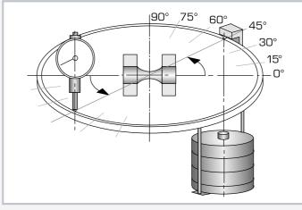
Clamped specimen:  $O^\circ$  = pure bending,  $9O^\circ$  = pure torsion, all angle settings between = combined loading
