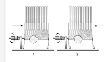
How adjustment of the bearing shell (bearing gap width) works: 1 bearing shell in right-hand position, 2 bearing shell in left-hand position
