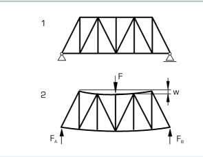
Bend test on a plane truss SE 100.04; 1 unloaded truss, 2 loaded truss, F test load,  $F_{\rm A}$  and  $F_{\rm B}$  support forces, w bending
