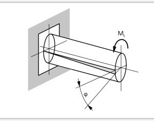
Principle of operation of torsion test:  $M_t$  twisting moment,  $\phi$  twisting angle
