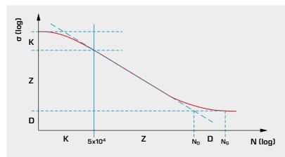
N load cycles, o stress load, K short-term strength, Z fatigue strength, D endurance strength,  $N_D$  number of load cycles from endurance strength is given, N<sub>G</sub> limit load cycles
