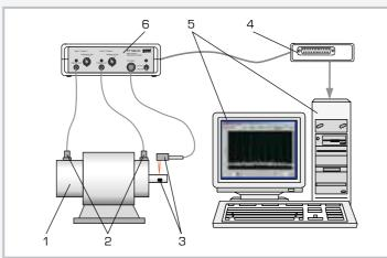
1 vibrating machinery, 2 acceleration sensors, 3 shaft with reference sensor, 4 USB box, 5 PC (PC not included), 6 measuring amplifier / filter
