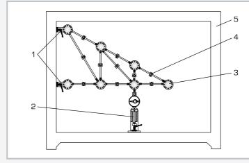
1 support, 2 load application device with force gauge, 3 node disk, 4 bar with measuring point, 5 frame SE 112  $\,$
