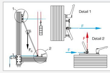
1 movable support, 2 fixed support;  $F_G$  applied force; red: cable with weights, compensates the vertical support force, blue: cable with weights, compensates the horizontal support force
