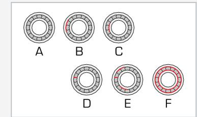
A) undamaged bearing, B) bearing with damage to outer race, C) bearing with damage to inner race, D) bearing with damage to a roller body, E) bearing with damage to roller body, outer and inner race, F) heavily worn bearing
