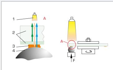
Determine the thickness of the lubricating film by optical interference: 1 halogen lamp, 2 glass plate with dielectric coating, 3 lubricating film, 4 steel sphere; arrows orange: incident light, green: dielectric coating reflects 30% of the light, blue: steel sphere reflects the remaining light
