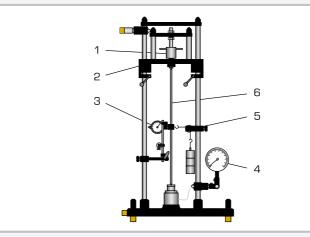
1 spindle, 2 height-adjustable load member, 3 dial gauge for lateral deflection of the test bar, 4 dynamometer, 5 mechanism for generating a lateral load, 6 test bar
