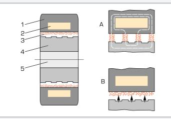
Principle of operation of a magnetic particle brake: 1 stator, 2 exciter coil, 3 gap with magnetic particles, 4 rotor, 5 shaft, A current flows: magnetic particles connect rotor and stator, resulting in friction and braking, B current flow interrupted: magnetic particles are pressed against the stator by centrifugal force, and the rotor can rotate
