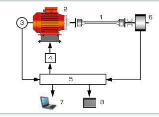
1 specimen, 2 gear motor, 3 incremental encoder, 4 frequency converter, 5 microprocessor, 6 strain gauge measuring shaft, 7 PC, 8 touch panel
