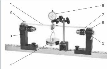
1 beam, 2 clamp fixing for bending test, 3 support block, 4 weight, 5 device to generate twisting moment in the torsion test, 6 support for bending test, 7 clamping chuck for torsion test, 8 dial gauge
