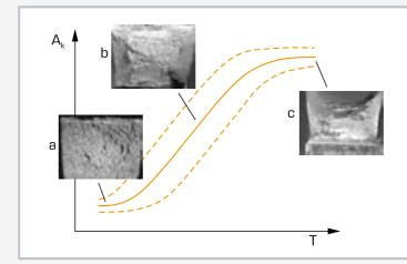
Notched bar impact work-temperature diagram with typical fracture surfaces: average-value curve with distribution area,  $A_k$  notched bar impact work, T temperature; a depth position with low-deformation fractures, b transition region (steep front) with mixed fractures, c height position with ductile fractures
