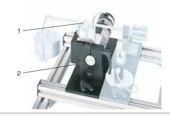
1 TM 260.03 experimental unit studies a tribological system, consisting of a pin and disk, which slide against each other, 2 TM 260 drive unit
