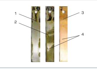
Experimental result: a steel specimen (2) and a copper specimen (3) were electrically connected (4) and supplied with an external voltage. A steel specimen (1) with no electrical connection was used as a reference.
