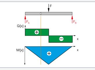
Shear force and bending moment diagram on beam with mid point load: line (orange): position of the hinge at which the internal forces of the beam are indicated
