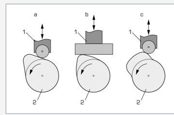
1 engaging member (rolling receiver with plunger / flat receiver with plunger), 2 camshaped cam member; a tangent cam with roller plunger, b circular arc cam with flat plunger, c hollow cam with roller plunger
