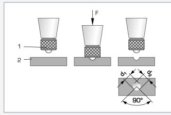
Brinell hardness test: 1 hardened steel ball, 2 specimen; F test load, d1 and d2 dimensions of the impression surface
