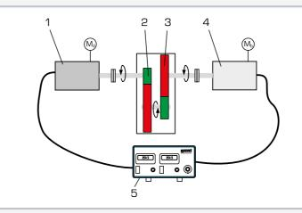
Determining the efficiency in the 2-stage spur gear: 1 motor, 2 first stage, 3 second stage, 4 brake, 5 display and control unit;  $M_d$  drive torque,  $M_b$  braking torque
