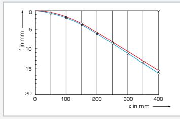
Elastic line of a cantilever beam: f draw down, x distance; red: calculated values, blue: measured values
