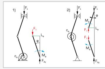
$\begin{array}{l} 1) \mbox{ experimental setup for elastic support} \\ 2) \mbox{ experimental setup for elastic joint;} \\ F_k \mbox{ buckling force, } F_1 \mbox{ articulation force, } F_{Ay} \mbox{ support reaction,} \\ M_\phi \mbox{ internal bending moment, } L_\phi \mbox{ deflection, } c_\phi \mbox{ torsional rigidity,} \\ \phi \mbox{ deflection angle} \end{array}$
