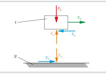
Forces occurring in dynamic friction: 1 friction body, 2 supporting friction surface; F  $_{G}$  weight, F  $_{H}$  tensile force, F  $_{R}$  friction force, F  $_{N}$  normal force
