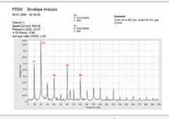
Envelope analysis on crank drive with clearance at 600min<sup>-1</sup>. Dominant is the 2 <sup>nd</sup> order 2n with harmonic waves 4n, 6n, 8n etc.
