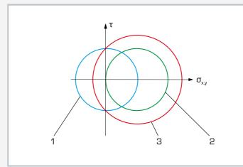
Mohr's circles for combined loading: bending with simultaneous torsion; 1 pure torsion, pure bending, 3 bending and torsion together;  $\sigma$  direct stresses,  $\tau$  shear stresses
