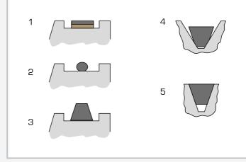
Comparison of different belt types: 1 flat belt, 2 cable, 3 V-belt, 4 adverse belt seat in the groove, 5 optimum belt seat in the groove
