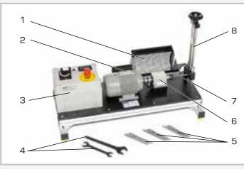
1 protective cover, 2 electric motor, 3 switch box, 4 tool, 5 specimens, 6 bearing, 7 clamped specimen, 8 load application device with spring balance and hand wheel
