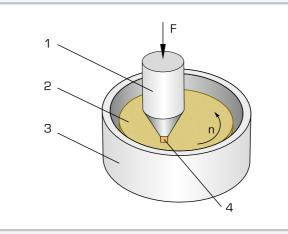
Tribological system pin and disk: 1 pin as counter body, 2 rotating disk as main body, 3 cup with lubricant as intermediate substance, 4 contact area; F force, n speed
