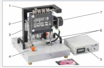
1 piston, 2 cylinder, 3 crankshaft, 4 foundation plate, 5 display and control unit, 6 force sensor, 7 drive motor
