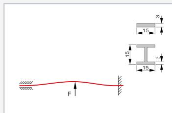
Plastic deformation of a beam, both beam profiles included in the scope of delivery
