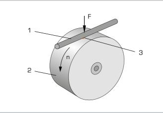
Tribological system of cylindrical pin and roller (point contact): 1 fixed cylindrical pin as counter body, 2 rotating roller as main body, 3 lubricant as intermediate substance; F force n speed
