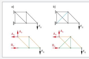
a) statically determinate truss, b) statically overdeterminate truss; red: support reactions, black: applied force, blue: surplus bar, green: compession bars (struts), orange: tension bars (ties)
