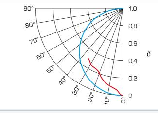
Movement of the shaft centre point during operation or startup behaviour, blue: theoretical semicircle curve, red: measuring results of TM 290; & relative lubricating film thickness
