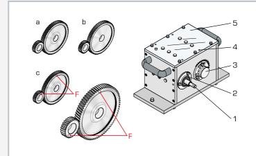
1 shaft end, 2 bearing cover with shaft gland, 3 bearing cover with centre distance adjustment facility, 4 tapped hole for vibration sensor, 5 transparent gear unit cover; a helical gear set, b spur toothed gear set, 4 damaged gear sets; F fault
