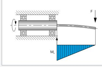
Functional principle of a fatigue strength test: cantilever mounted rotating specimen, loaded with a single force; F force, M<sub>b</sub> bending moment
