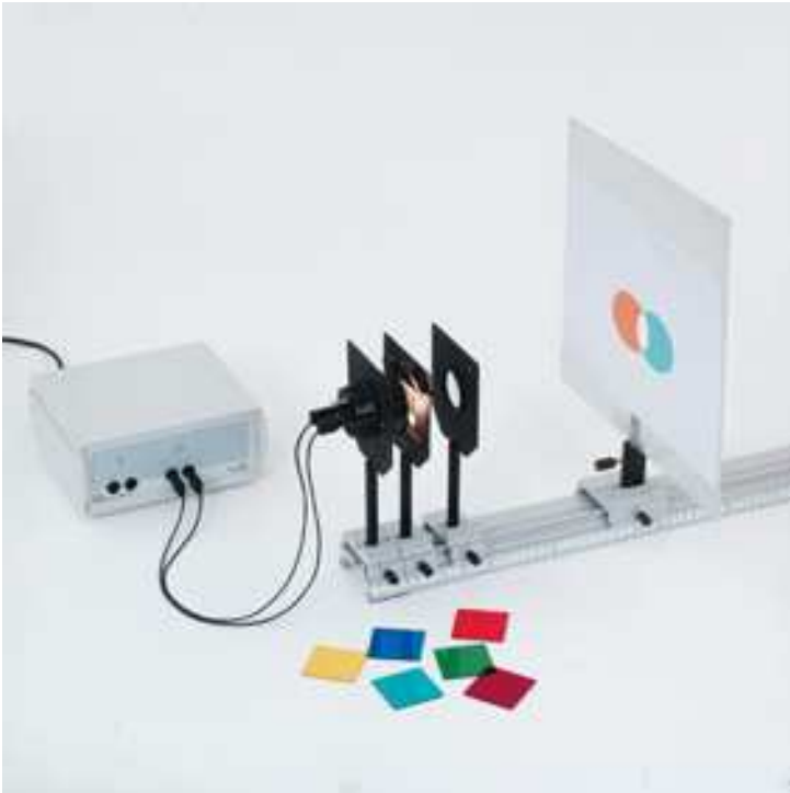
Determining the complementary colors by additive color mixture.
