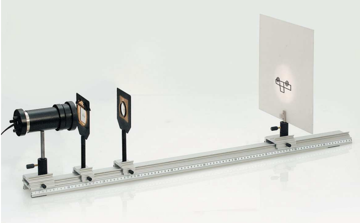
Confirmation of the lens equation.
