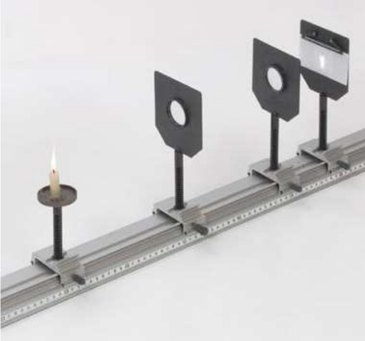
Demonstrating the principle of operation of a zoom lens.
