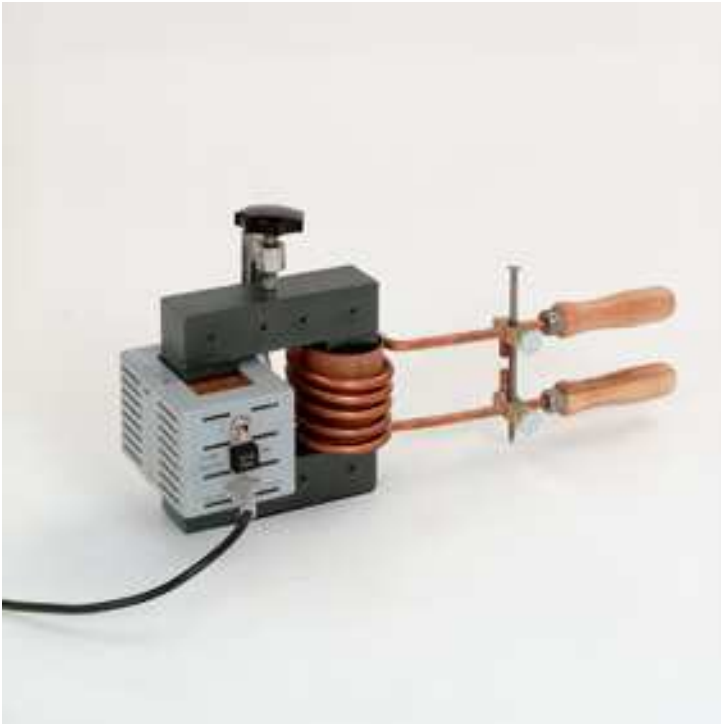
Demonstrating the heating effect of a high-current transformer.
