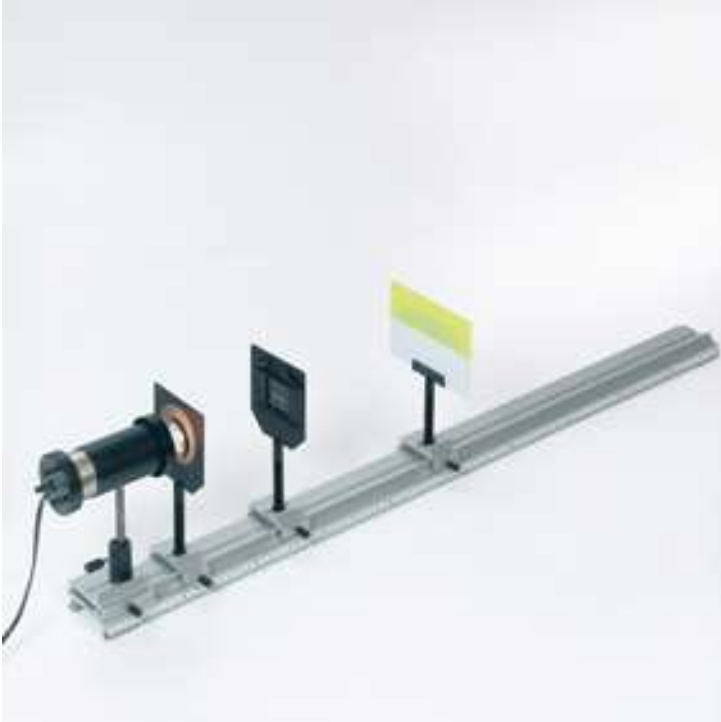
Detection of ultraviolet radiation by means of an ultraviolet phosphorescent screen.
