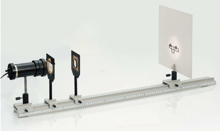
Determination of the focal length of a convex lens.
