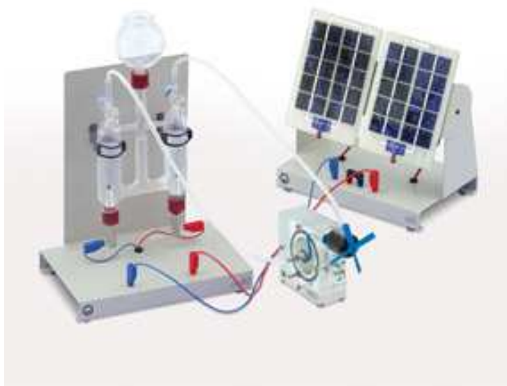
Demonstrating the transformation of energy in a fuel cell.
