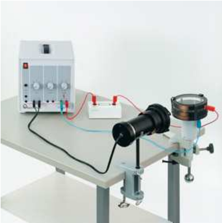
Demonstrating the trajectories of a particles in a Wilson cloud chamber
