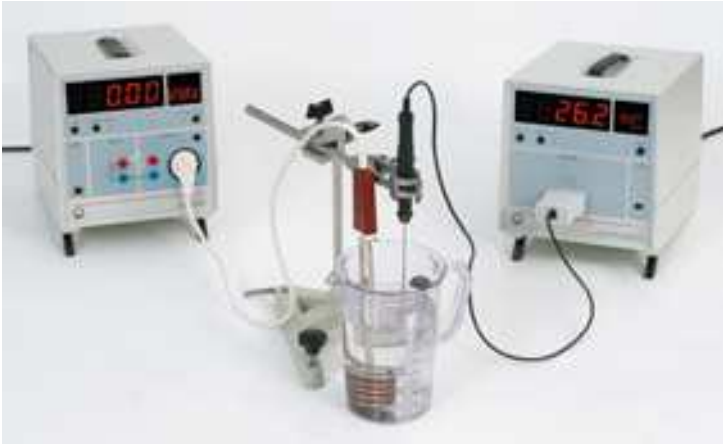
Determination of specific heat of water.
