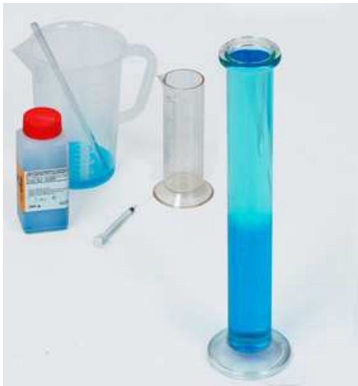
Demonstrating diffusion in copper sulphate and water.
