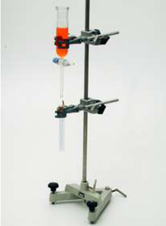
Determining the volume of a drop of water.
