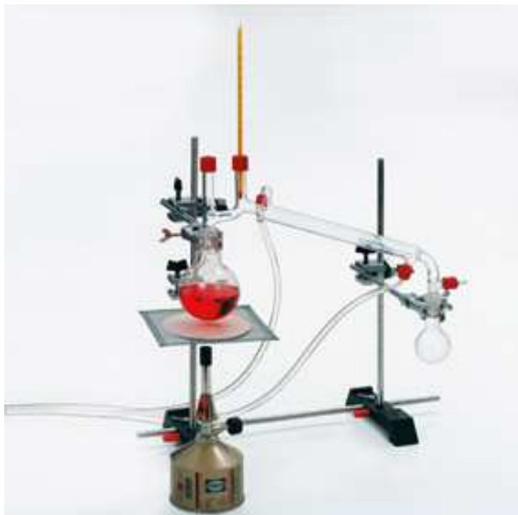
Demonstrating the isolation of strong alcohol by distilling red wine.
