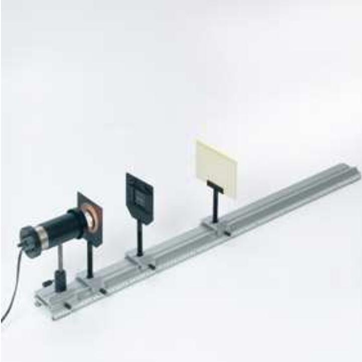
Detecting infrared radiation by means of a zinc sulphide screen.
