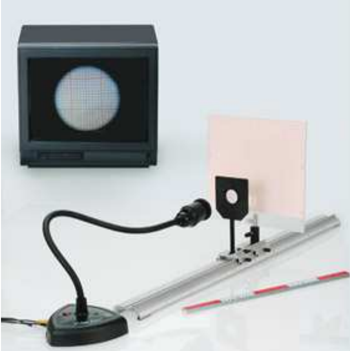
Determination of the magnification V_L of a magnifier.
