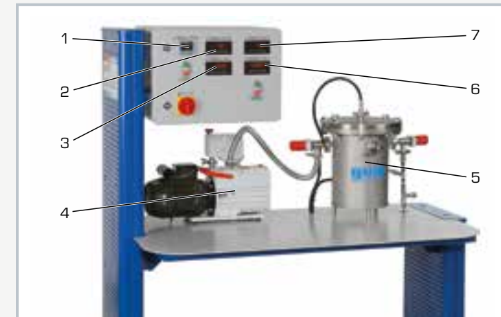
1 temperature controller with temperature display, 2 temperature display, 3 power display, 4 vacuum pump, 5 pressure vessel, 6 vessel's absolute pressure display, 7 vessel's relative pressure display
