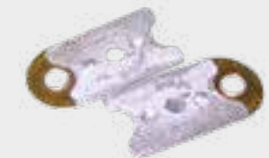
Trip element with melted solder joint
