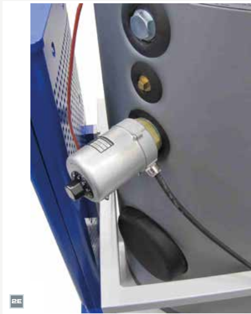
HL 320.02 heater installed in the bivalent storage tank of HL 320.05
