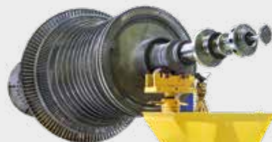
Disassembled steam turbine rotor
