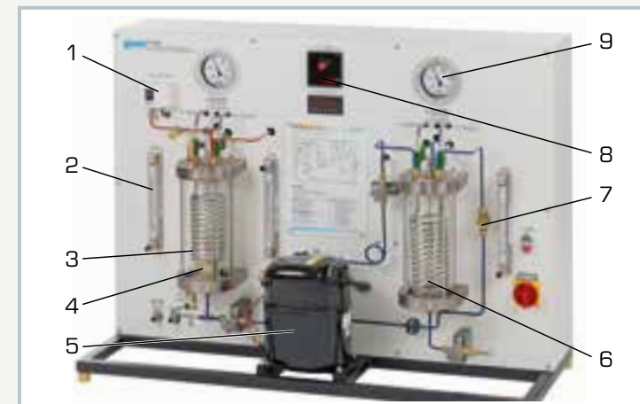
1 pressure switch, 2 flow meter, 3 condenser, 4 expansion valve, 5 compressor, 6 evaporator, 7 sight glass, 8 temperature display, 9 manometer
