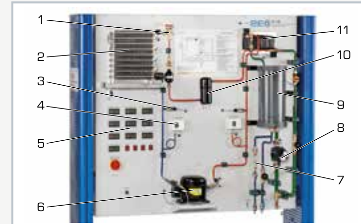
1 expansion valve, 2 evaporator with fan, 3 pressure sensor, 4 pressure switch, 5 displays and controls, 6 compressor, 7 cooling water flow meter, 8 pump, 9 hot water tank, 10 receiver, 11 cocondenser
