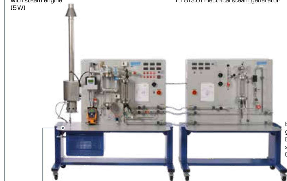
ET 813 Two-cylinder steam engine (500W) together with HM 365 Universal drive and brake unit and ET 813.01 Electrical steam generator
