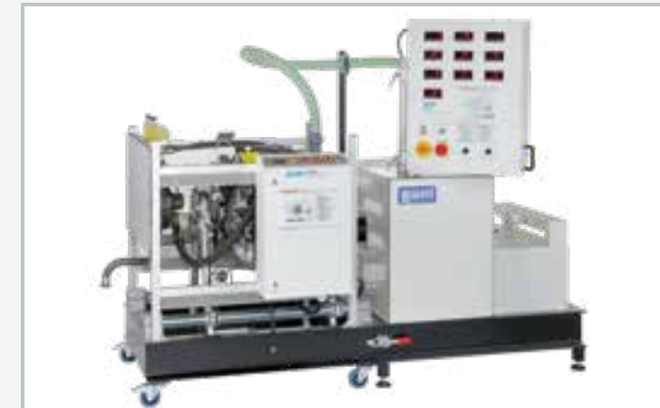
The illustration shows the CT 400 in conjunction with the CT 400.02 diesel engine.
