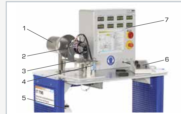
1 mixing pipe, 2 jet engine, 3 turbine platform, 4 force sensor for thrust measurement, 5 fuel tank, 6 gas turbine controls, 7 switch cabinet
