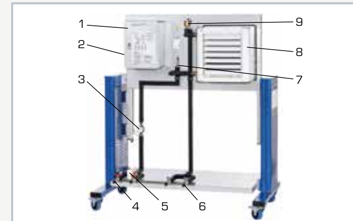
1 junction box, 2 CAN-bus connecting sockets, 3 flow meter, 4 feed flow, 5 3-way mixing valve, 6 return flow, 7 temperature sensor feed flow, 8 fan convactor, 9 vent valve
