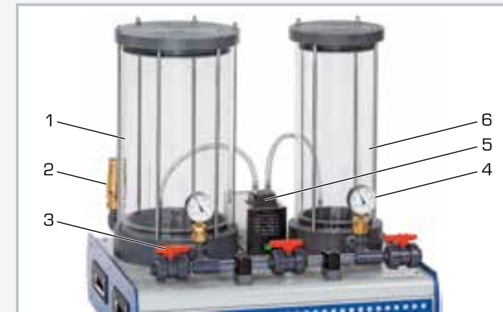
1 positive pressure tank, 2 safety valve, 3 ball valve, 4 manometer, 5 compressor, 6 negative pressure tank
